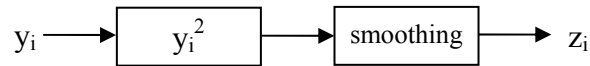
Figure 1. The envelope containing the profile of the spectrum area A_i is obtained by squaring the channel y_i and smoothing the result.
